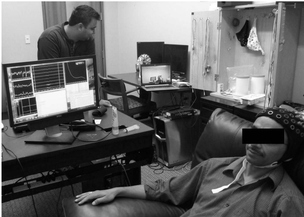
Figure 2. EEG Set-Up. EEG signals being recorded from a subject (the “Sender”) as the subject watches the computer game (the game screen is to the left and not shown in the picture). The larger screen displays EEG signals processed by the BCI2000 software. The smaller laptop screen placed further away is from the live Skype session and shows a “Receiver” subject in the TMS lab across the University of Washington campus. (Image from the pilot study referred to in the text). doi:10.1371/journal.pone.0111332.g002
